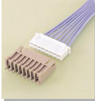
The header is tall and fully shrouded so as to prevent the resin used to coat the PC board coming into contact with the mating pins. Designed for use specifically with resin coated ("potted") PC boards.
