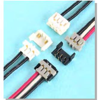
This ADH connector is compact and low profile type, height 1.9mm and width 4.3mm, 1.3 pitch wire-to-board connector.
