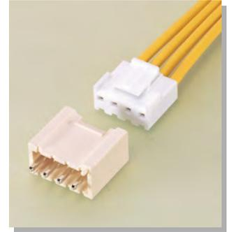
The header is tall and fully shrouded so as to prevent the resin used to coat the PC board coming into contact with the mating pins. Designed for use specifically with resin coated ("potted") PC boards.
