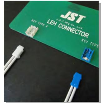
Considering about the luminescence property of LED package and the mating operability, this LEH connector is designed as low profile type connector for LED lighting, and achieves the space saving.. In consideration of connector mating operation to the LED mounting PCB that is integrated in the equipment, side-feed mechanism that provides to enable mating the connector from right above is adopted, and secure lock and mechanism for preventing wrong insertion are provided.
