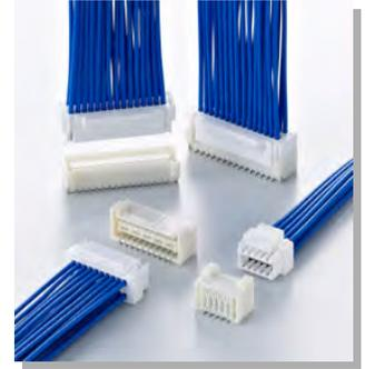
In order to correspond to the high-density PCB designing, this ZPD connector is designed as 1.5mm pitch double row type connector with secure locking device.
