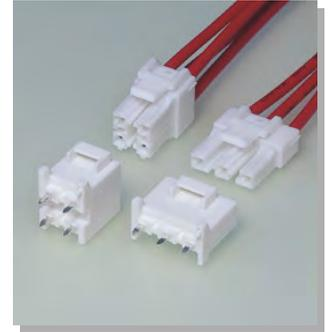
This connector is designed for wire-to-board 6.5mm pitch connector corresponding to large current. Secondary retainer, which prevents from insufficient insertion of contact and coming off contact, may use and large current circuit can be connected certainly and safely.
