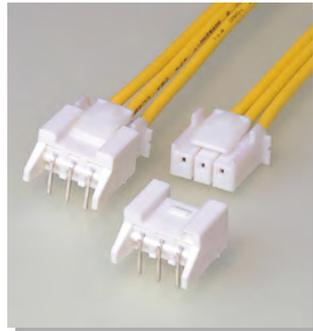
VU connector is small type 3.96mm pitch PC board connector for large current and has the high reliability in a power supply circuit, considering the fully shrouded connector header structure against "vibrating connector" and "distorted extraction".
