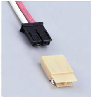
Low profile connector with high withstanding voltage, designed for connecting liquid crystal display backlight lamps to their starters. The BHL connector is 2.8mm thick, so the mounting height is only 3.0mm.
